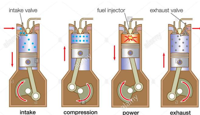
Figure 1: Diagram detailing the 4 stages of a 4-stroke internal combustion engine.
